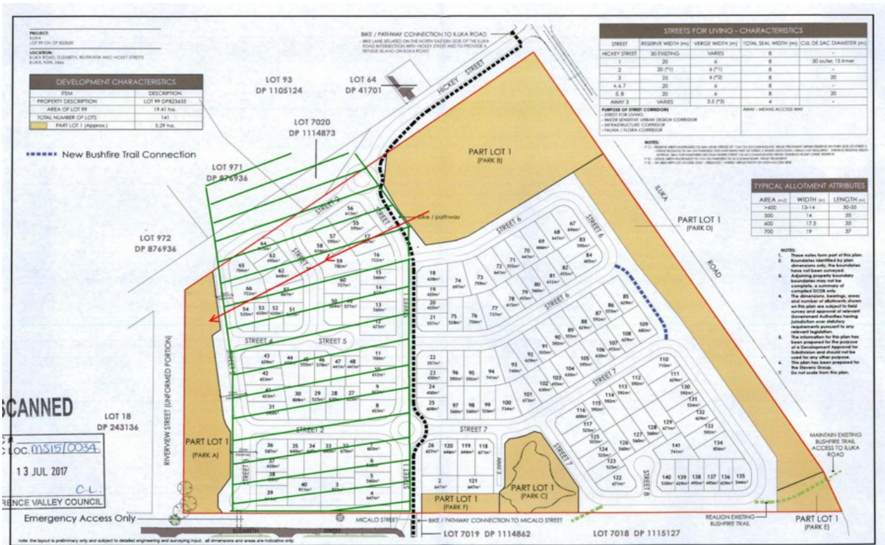
Green hatching shows the minimum width of the broken wildlife movement corridor
